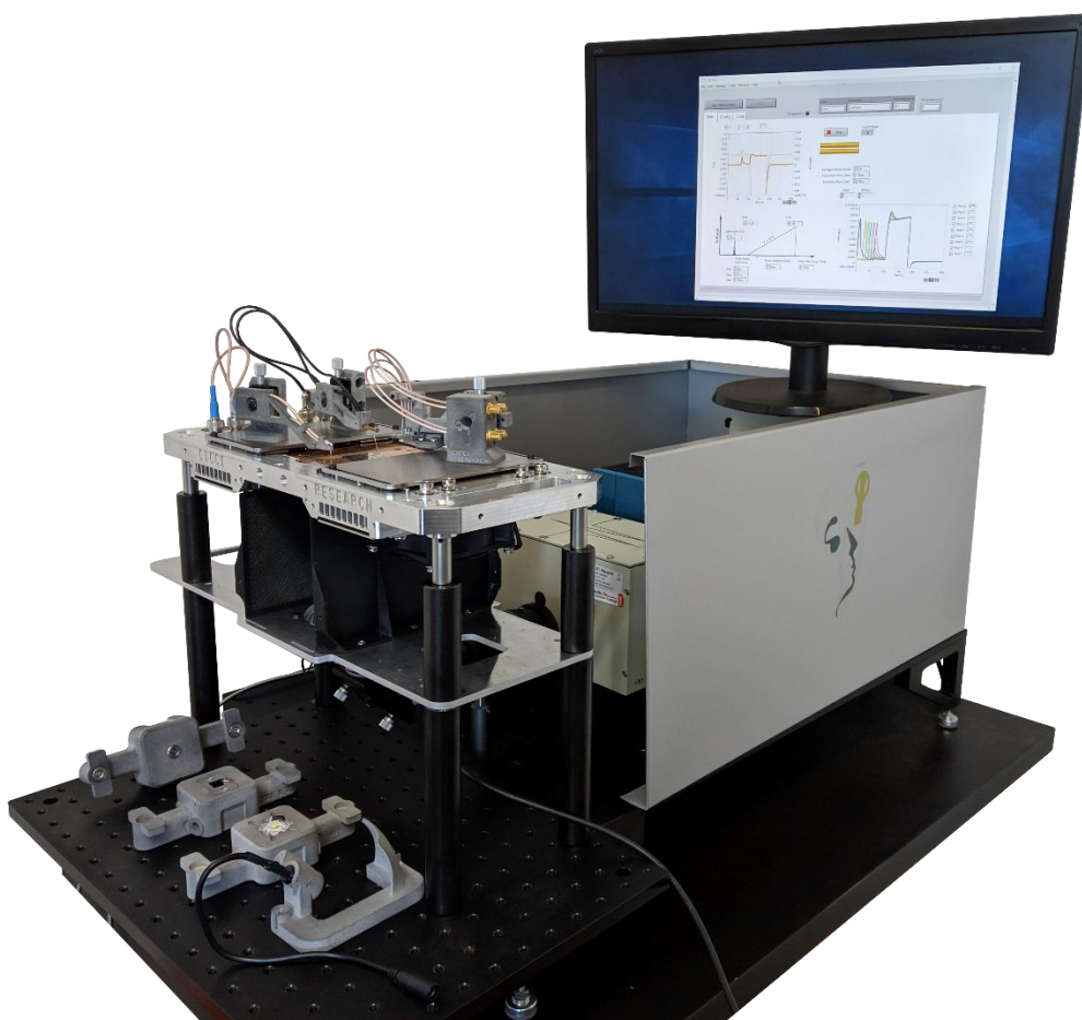
Figure 3 – Overview of a complete system showing the thermal stage, a monochromatic line, and several accessories.
