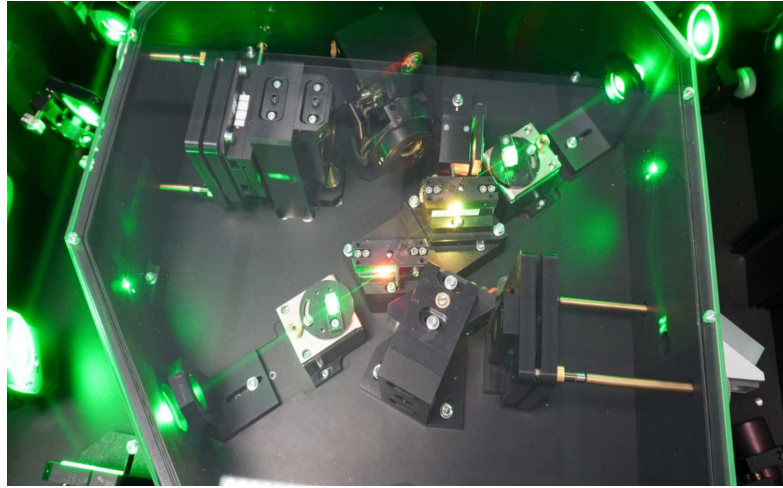
Figure 2.10: Sirah Credo Ti:Sa 10 kHz cavity
