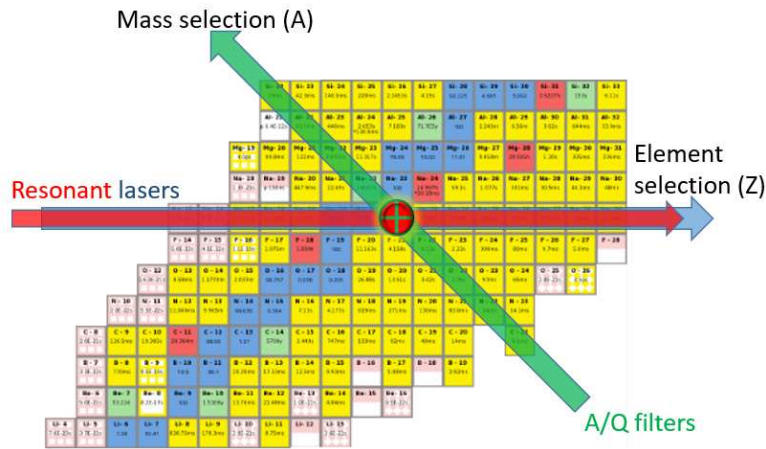
Figure 3.3: Principle of production of an isotopic beam with RILIS technique. The red-filled circle (with green cross-hairs) represents the isotope selected.
