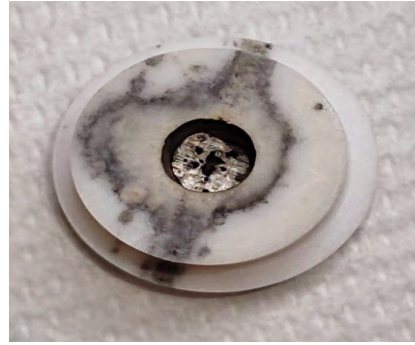
Figure 4.7: Teflon target holder with the silver target
