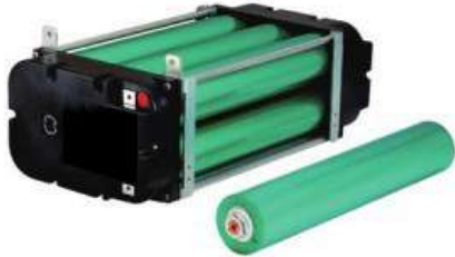
Figure 48 test module Li/Mn.
