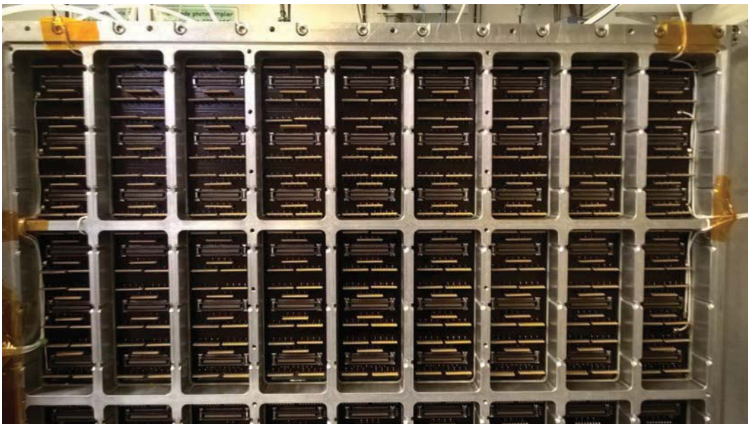
FIGURE 7.34: The Micromegas PCB (back view) after attaching the resistances;
