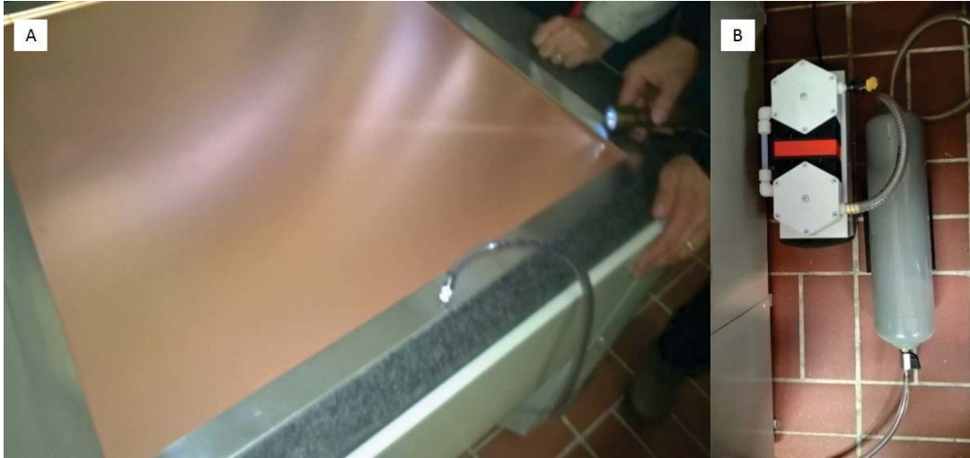
FIGURE 6.3: A. The frame by which the PCB foil had been pressed onto the marble top of the thickness measuring machine. B. The vacuum pump
