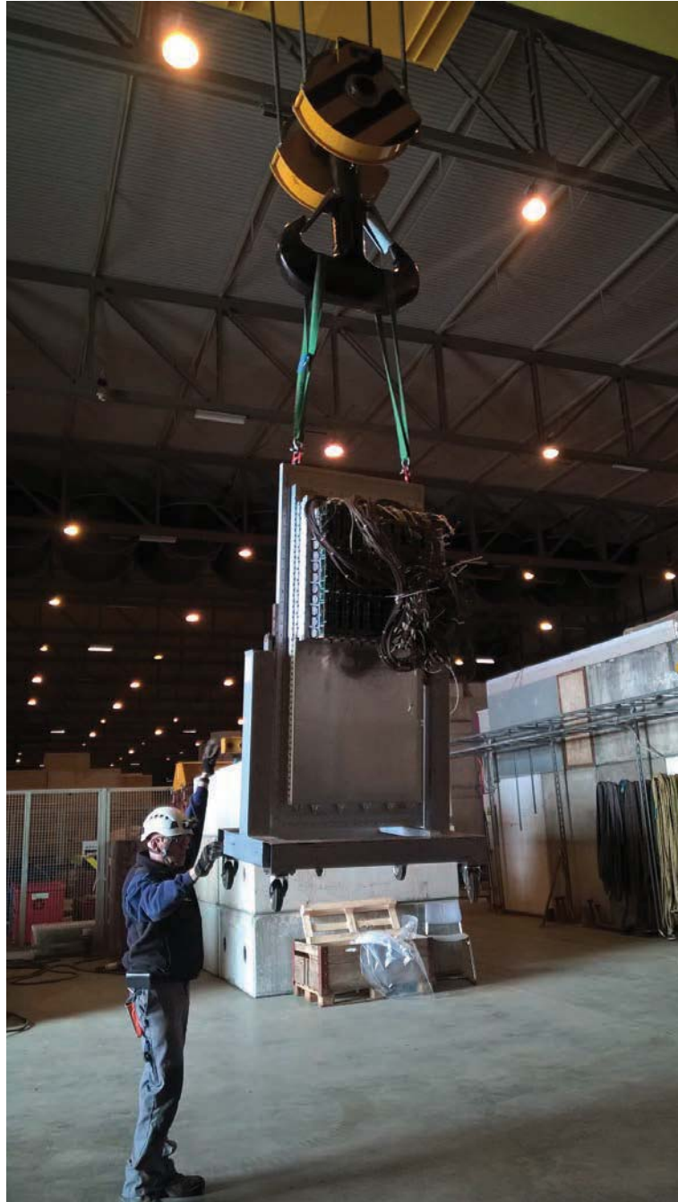
FIGURE 7.56: Craning up the modified new frame with MAPMTs for transportation from the clean room to the area.
