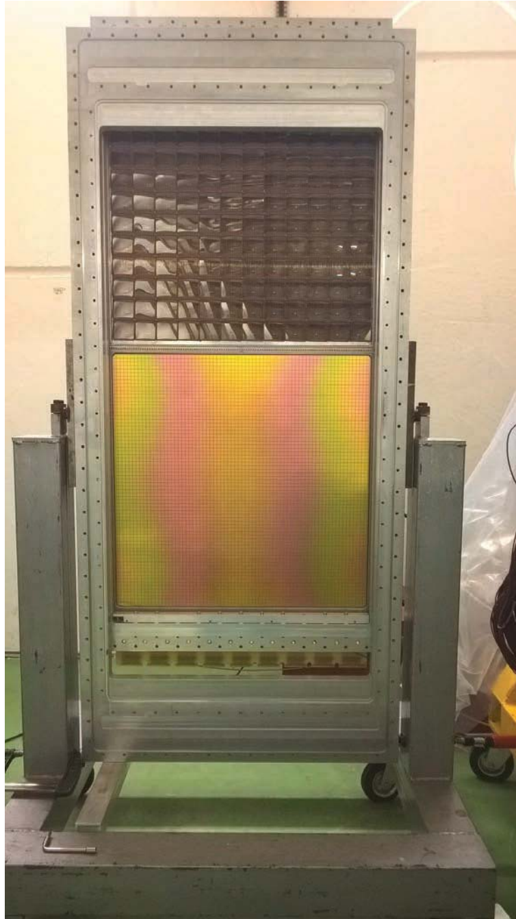
FIGURE 7.53: The old frame with MWPC with CsI photo-cathode (bottom part) and MAPMTs with fused silica lenses (top part), in CERN clean room facility
