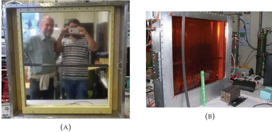
FIGURE 6.17: A. Assembled drift plane made with 300nm Al coated mylar foil. The reflected image of me and my supervisor can be seen. B. The large Kapton window of the 800 \times 800 \text{ mm}^2 allows to test the whole surface of the two MMs using the ^{55}\text{Fe} X-Ray source.
