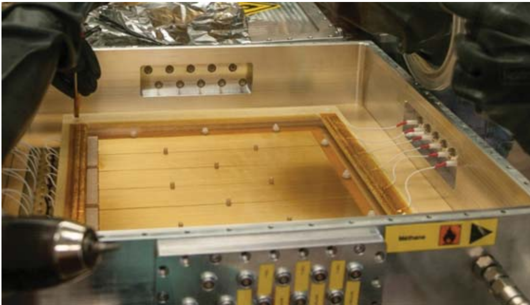
FIGURE 5.24: Picture of a 300 \times 300 \text{ mm}^2 THGEM mounted in a PD
