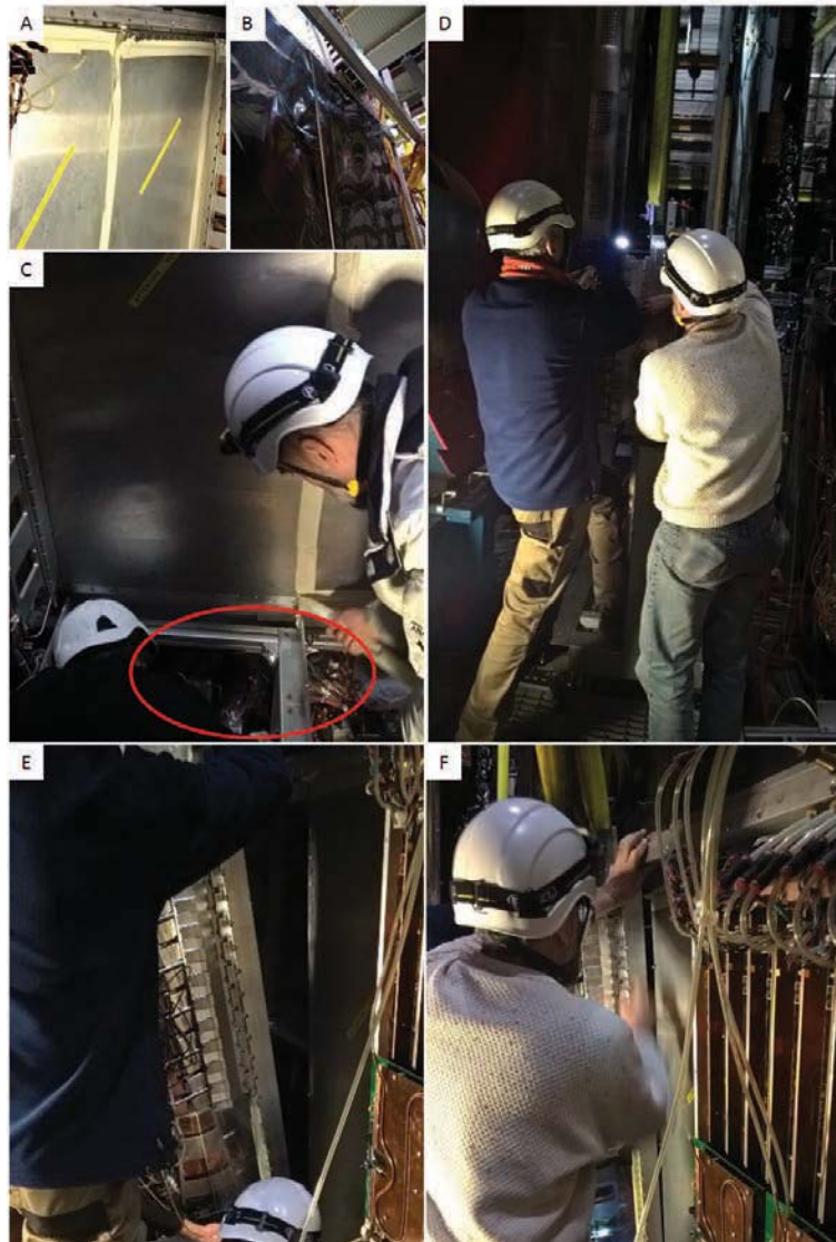
FIGURE 7.57: A: Fused Si Windows on COMPASS RICH-1 with protection cover. B: Fused Si windows after removing the protection. C: Special custom build support for mounting back PD frames with MAPMT system (marked with red circle). D, E and F: craning down of the PD frames with MAPMT system (D) and mounting on the RICH-1 (E and F)
