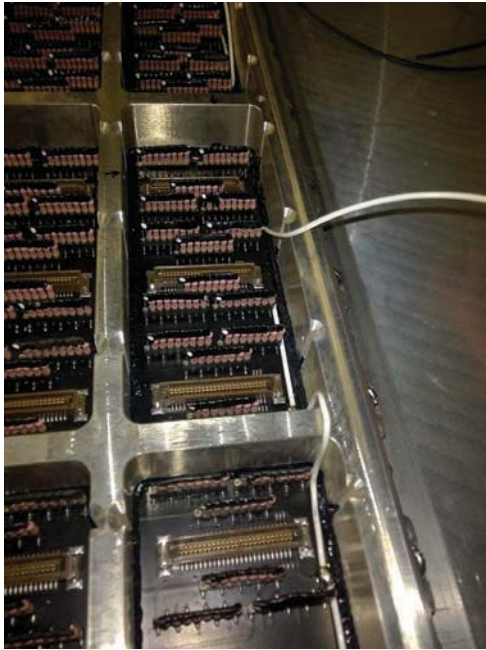
FIGURE 7.35: Particular of the hybrid frame equipped with final resistors and the black epoxy glue
