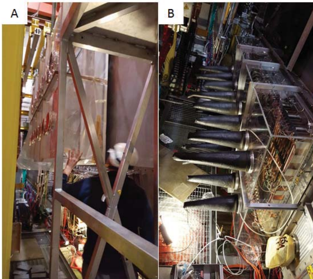
FIGURE 7.58: A: Craning Down the glove box to mount back the new hybrid PDs B: Glovebox in place flushed.
