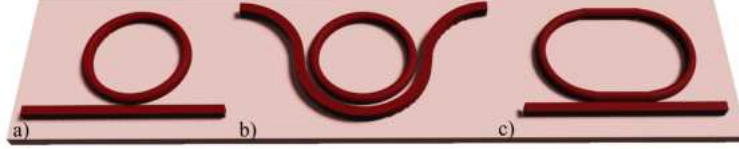
Figure 2.11: Sketch of microring resonator in All pass configuration for the point coupler (a), pulley (b), and racetrack (c) configurations.
