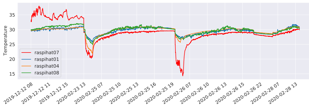
Figure 4.7: Sensor raspihat07 temperature values related to the prediction error outliers compared with the 3-nearest neighbours sensors.
