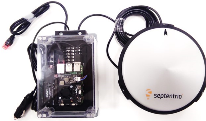
Figure J1.4: Final assembled system: Navigation EMERGE OBU
