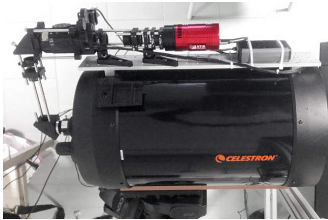
Fig. 4.5: The Celestron C11 telescope used in the horizontal atmospheric turbulence measurements. The optics are attached on a tray over the telescope.
