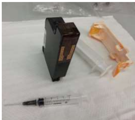
Figure 35. Ink-filled cartridge with precursor solution.
