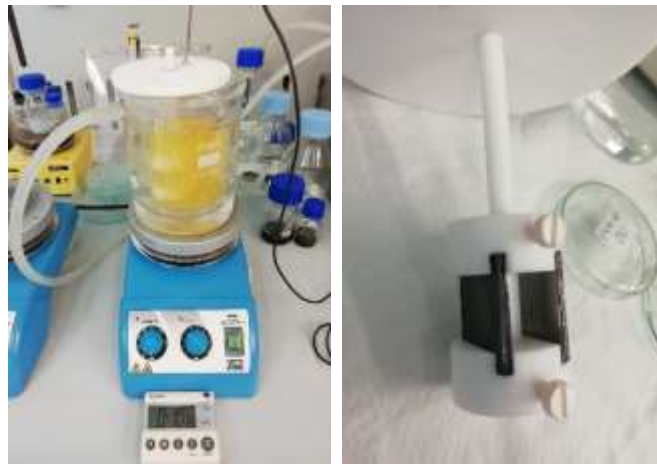
Figure 43. Two samples undergoing chemical bath for buffer layer deposition.
