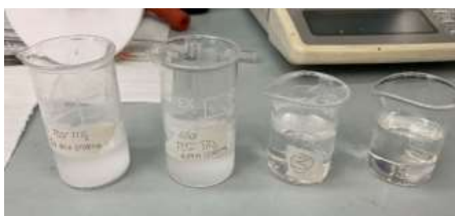
Figure 76. Samples of \text{TiO}_2 solution at different stirring times.
