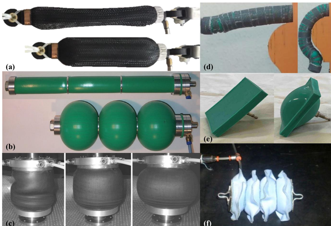
Figure 1.9 (a) McKibben muscle; (b) Straight fibers muscle; (c) Bi-directional actuator; (d) Bending pneumatic actuator; (e) Air-pocket; (f) Bellow muscle. [95]
