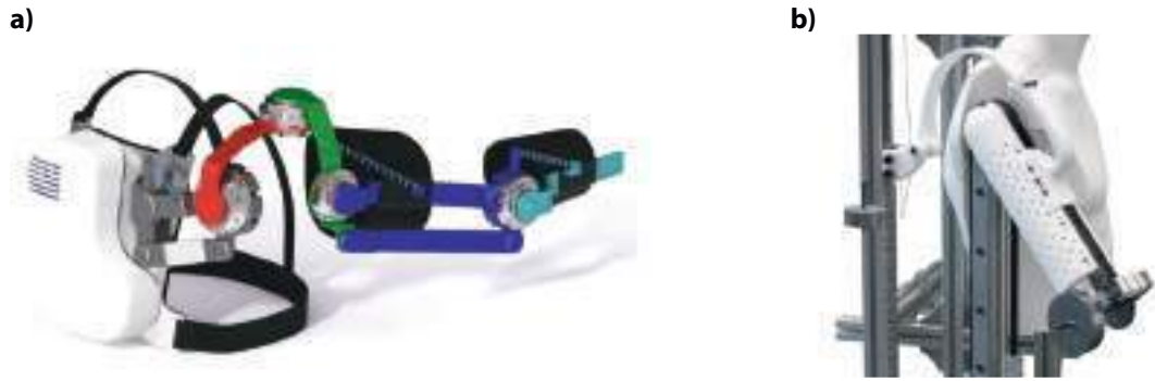
Figure 3.1: Upper limb exoskeletons examples from the literature with passive springs. a) 6-Degrees Of Freedom (DOFs) hybrid shoulder-elbow exoskeleton [30]. b) 1-DOF passive shoulder exoskeleton [31].
