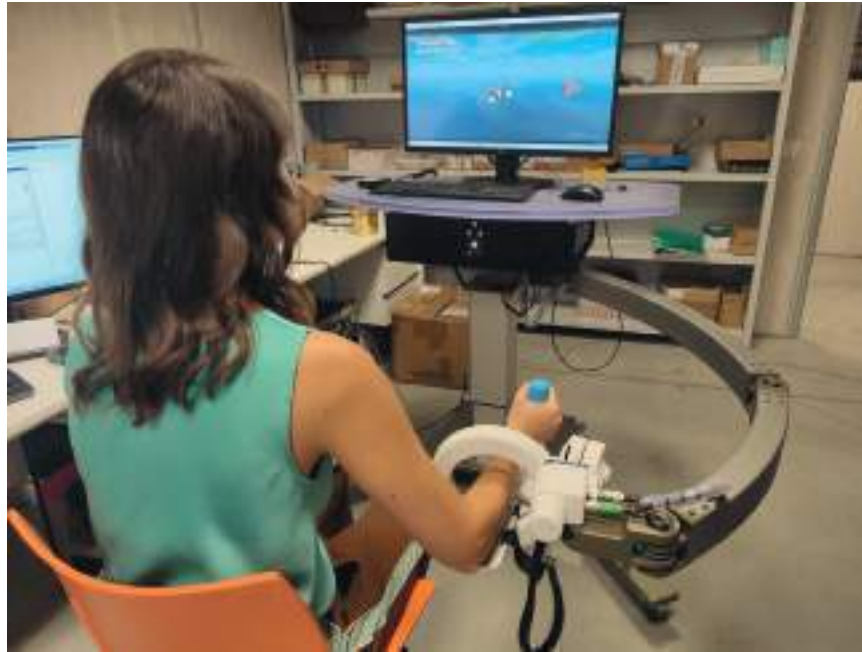
Figure 4.7: Experimental setup of the rehabilitation platform: subject wearing the wrist exoskeleton and performing the Flight Simulator serious game.
