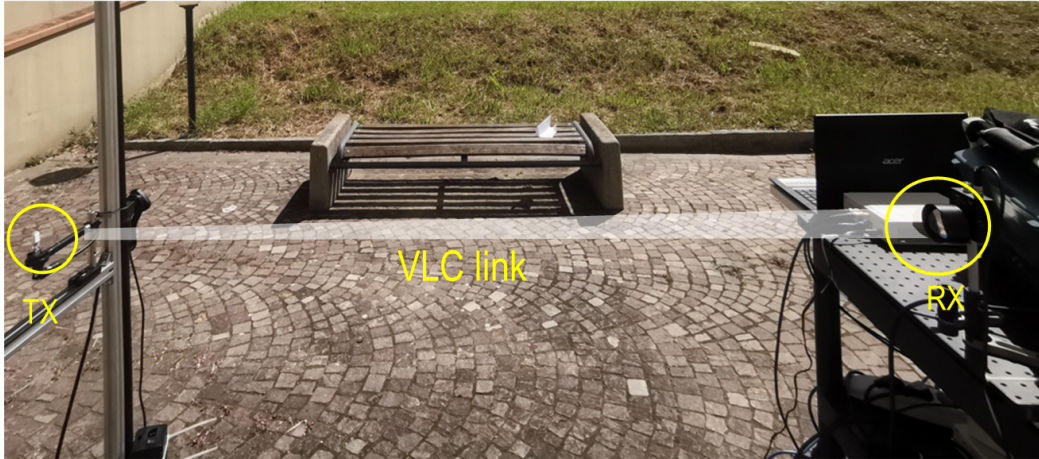
Figure 6.12: Outdoor measurements setup under strong solar irradiance.
