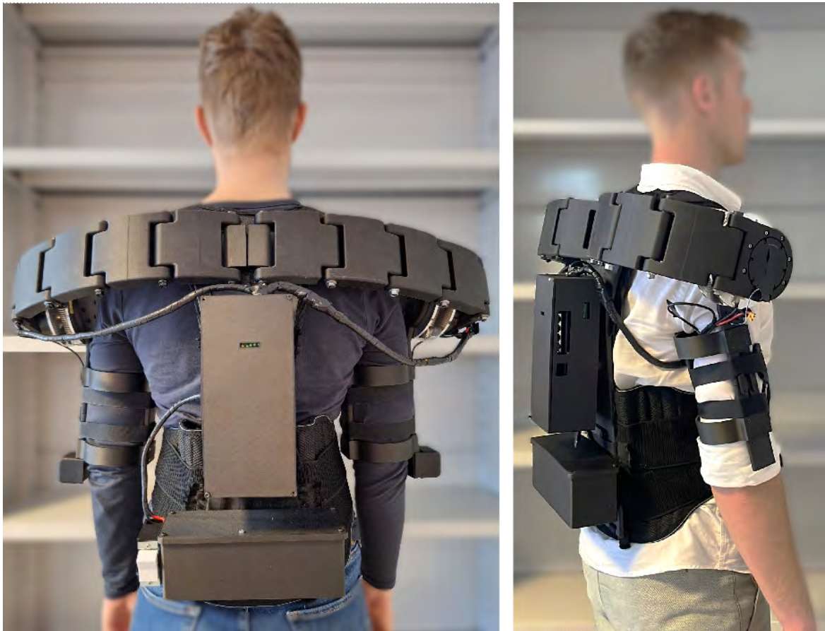
Fig. 2.1 The proposed Flexos exoskeleton for the shoulder.
