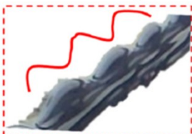
Fig. 3.6: Electromagnetic assistance to improve the printing quality, tested on the proposed soft ink (Ecoflex 00–10 +30 wt% of Fe_3O_4 ). a) Effect of different current inputs (0 A, 3.5 A, and 4.5 A) provided to the copper coils to generate electromagnetic force on the printing quality, and b) benefits of the proposed approach in overcoming over-extrusion problems when a layer height of 0.1 mm is set.
