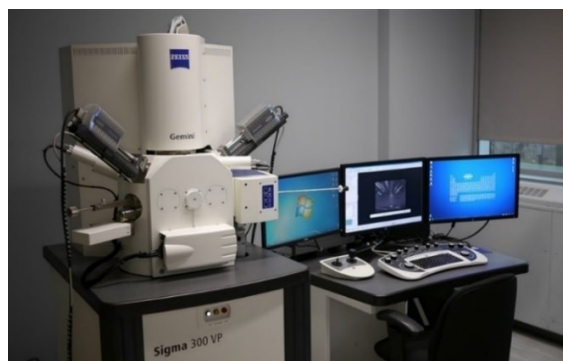
Figure 3.11: High-resolution Field Emission Scanning electron microscope (SEM), ZEISS Sigma 300 VP, used in the present thesis work. [163]
