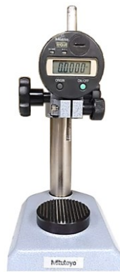
Figure 3.24: Mitutoyo Absolute comparator.
