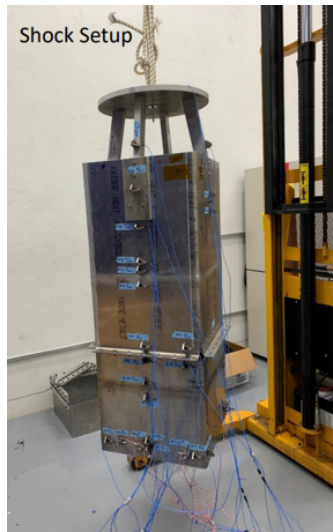
Figure 5.25: Shocksat Shock setup
