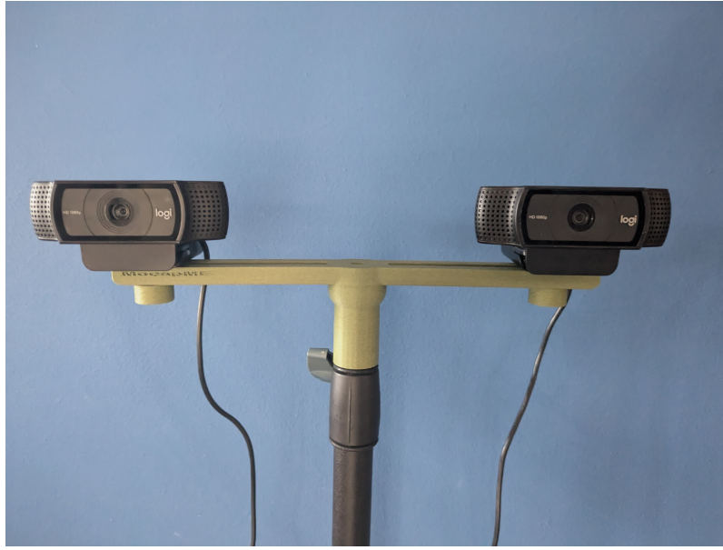
Figure 5.11: 3D camera setup with Logitech C920 cameras and rigid frame.
