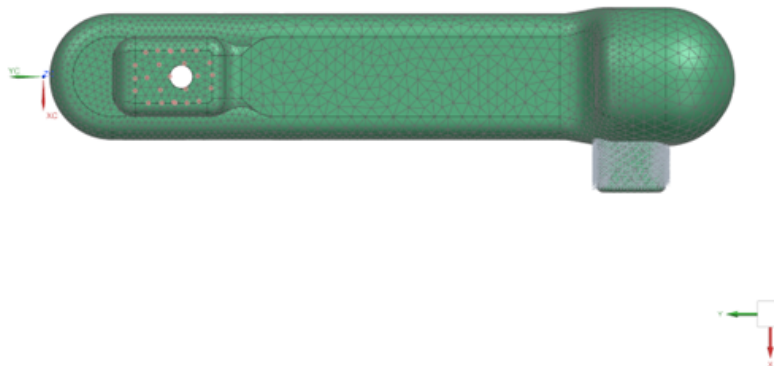
Figure 4.61: Loads and boundary conditions applied during Finite Element Analysis (FEA) of the torque wrench. Source: [45]
