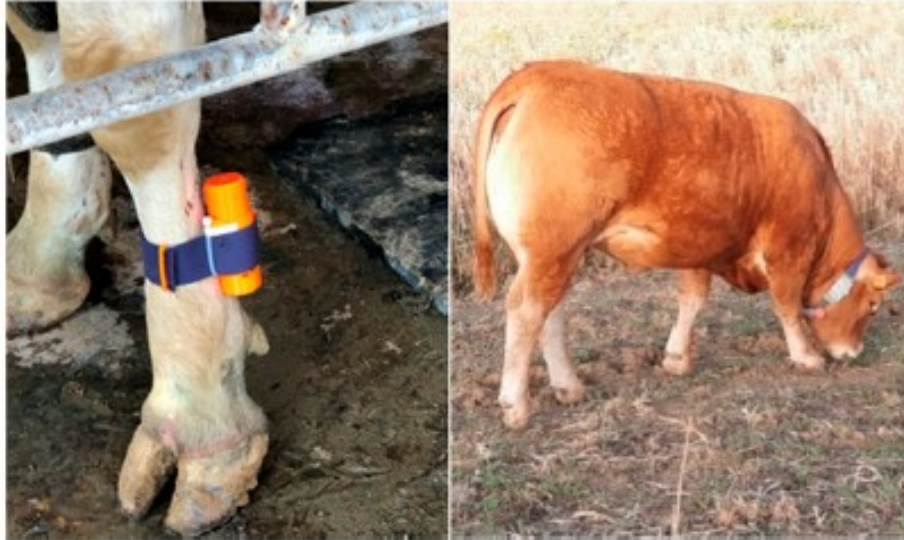
Figure 2.2: Example of pedometer and collar worn by cows [26, 93]
