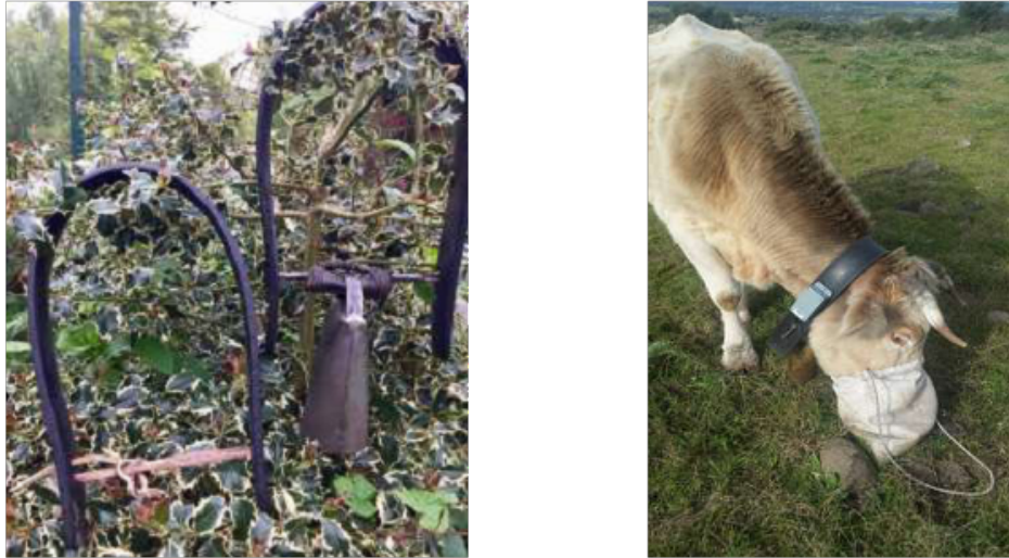
Figure 7.2: Low power-global positioning system device attached to the cow's collar.
