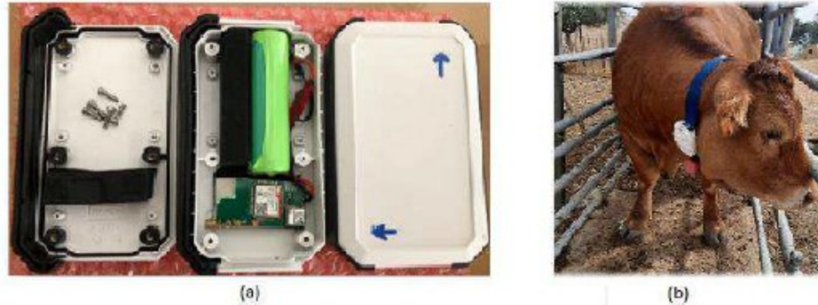
Figure 3.2: a) Customized device equipped with triaxial accelerometers b) Device attached to the cow collar.
