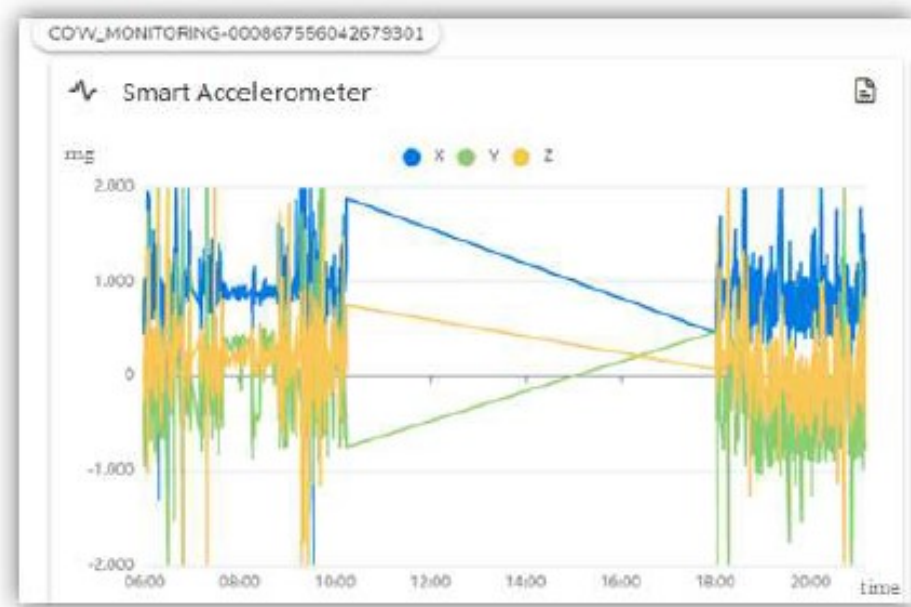
Figure 3.3: Graph of acquired data. To increase battery life the device entered in sleep mode from 10:00 a.m. to 17:59.
