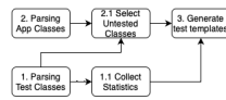
Figure 5.2: Flowchart representing the main steps followed by the approach generating test cases.
