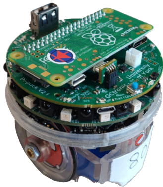
Figure 6.3: E-puck2 and two of its extensions mounted on it: range & bearing board and Pi-puck.
