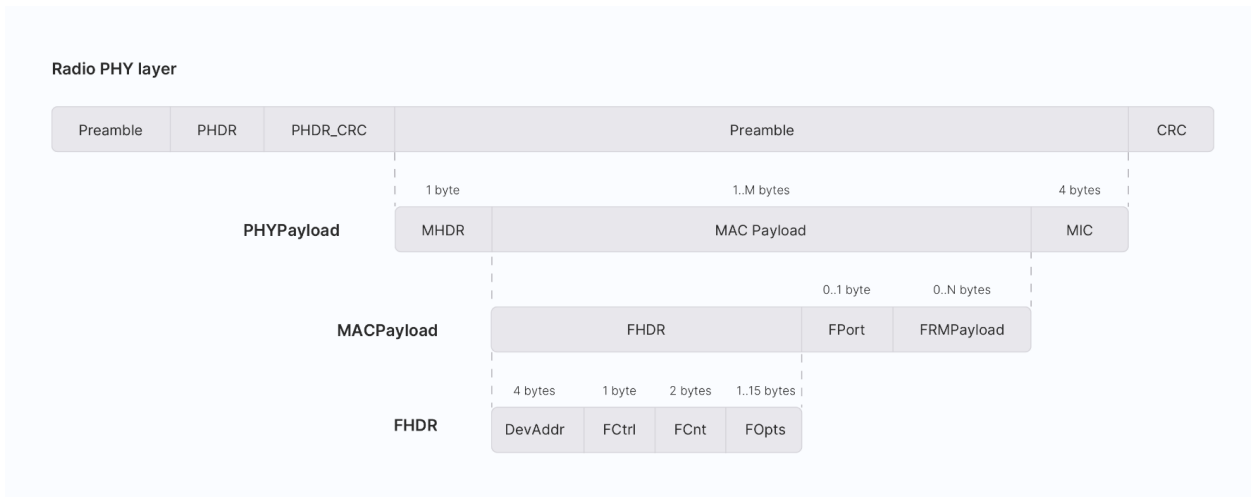
Figure 3.6: The structure of a LoRaWAN frame. Being built on top of LoRa, the physical layer has the structure of a LoRa frame. Its PHYPayload is then divided into MAC Header (MHDR), MAC payload, and a Message Integrity Code (MIC) to check the integrity of the whole packet. The MAC Payload contains application data, which again is divided into Frame Header (FHDR), FPort (used to distinguish different applications), and its payload
