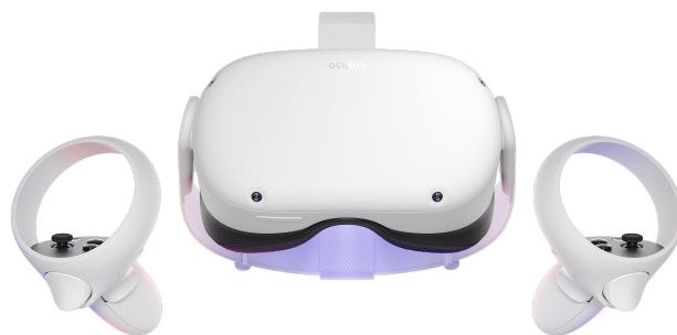
Figure 5.1: Meta Quest 2: headset and controllers
