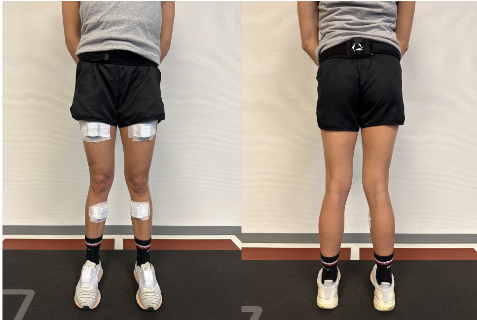
Figure 5.8: Placement of Sensors on Lower Limbs. This image shows the front and back views of sensor placement on the lower limbs. Sensors are affixed to key anatomical landmarks, including the thighs, shanks, and feet, to accurately capture motion data during gait analysis. Proper placement ensures reliable and consistent measurements for biomechanical evaluations
