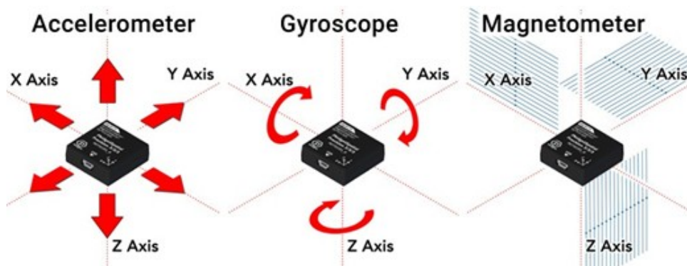
Figure 3.2: Components of an Inertial Measurement Unit (IMU). A diagram illustrating the three primary sensors within an Inertial Measurement Unit (IMU): the accelerometer, gyroscope, and magnetometer. The accelerometer measures linear acceleration along the X, Y, and Z axes, the gyroscope detects angular velocity or rotation around these axes, and the magnetometer provides orientation relative to the Earth's magnetic field. Together, these components enable precise motion tracking and spatial orientation in various applications
