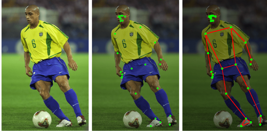
Figure 2.8: Markerless-based Motion Analysis framework. A sequence of images illustrating the application of markerless motion analysis. The first image represents the original scene; the second shows detected key body landmarks, and the third connects these landmarks to create a skeletal model. This approach leverages computer vision techniques to analyze human motion without physical markers, enabling efficient and non-invasive movement assessment in various settings. Adapted from [68]
