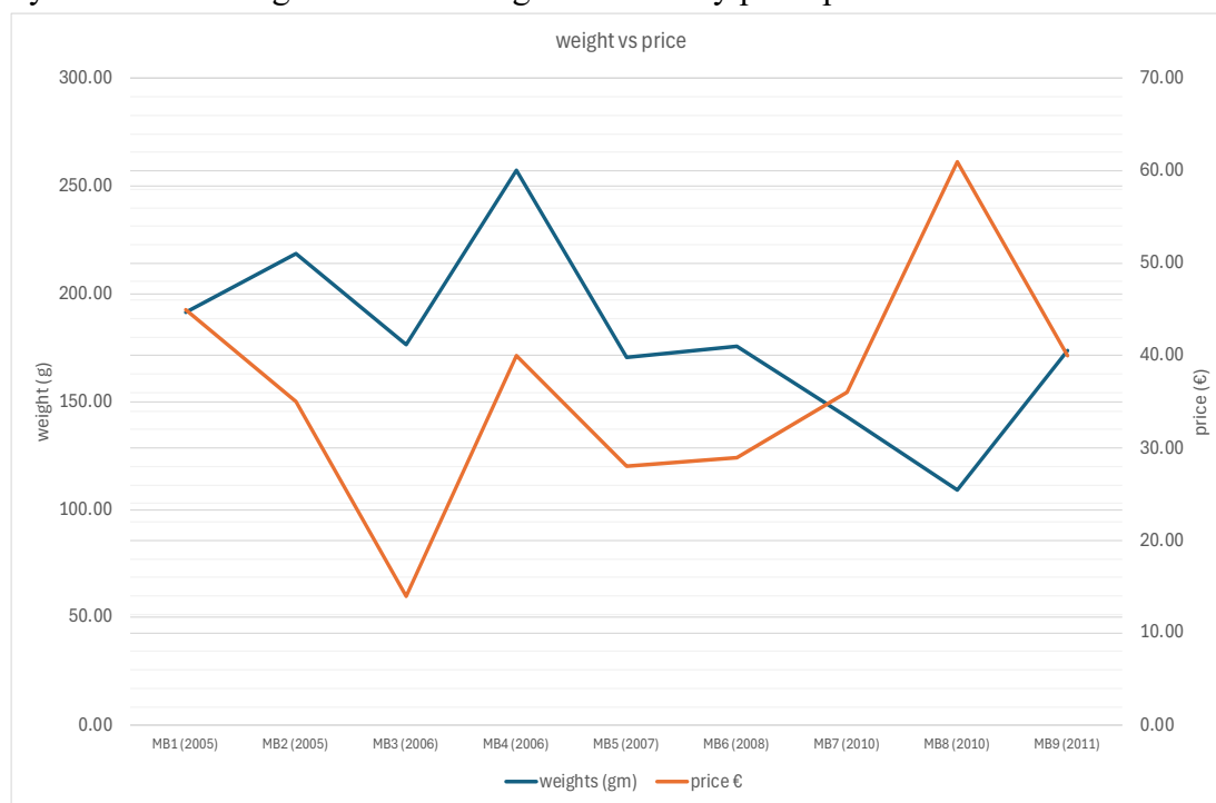
Figure 13. Visualization of the sampled motherboard PCB weights in grams and their current market value in Euros. Shown between brackets next to the name of each sample is the year of production
