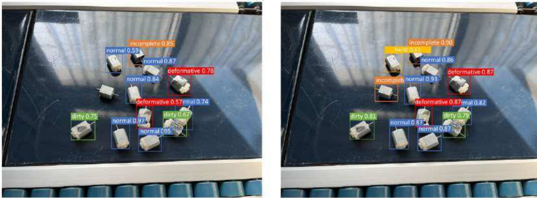
FIGURE 3.4: Surface imperfections Detection [15]
