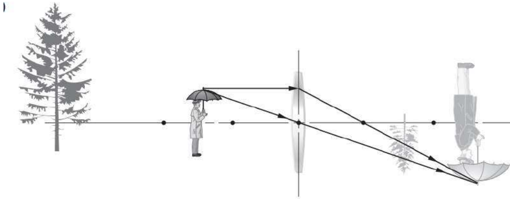
FIGURE 2.6: The image-forming behavior of a thin positive lens [10]
