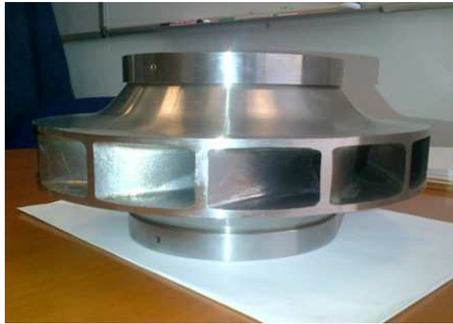
Figure 4.35: Outlet view of the 3D CAD and of the real impeller obtained by means of Lost-foam casting technology.
