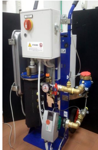
Figure 22 Pulsating TRT machine developed at the University of Genova and employed for the TRT experiment here described as Case#2.
