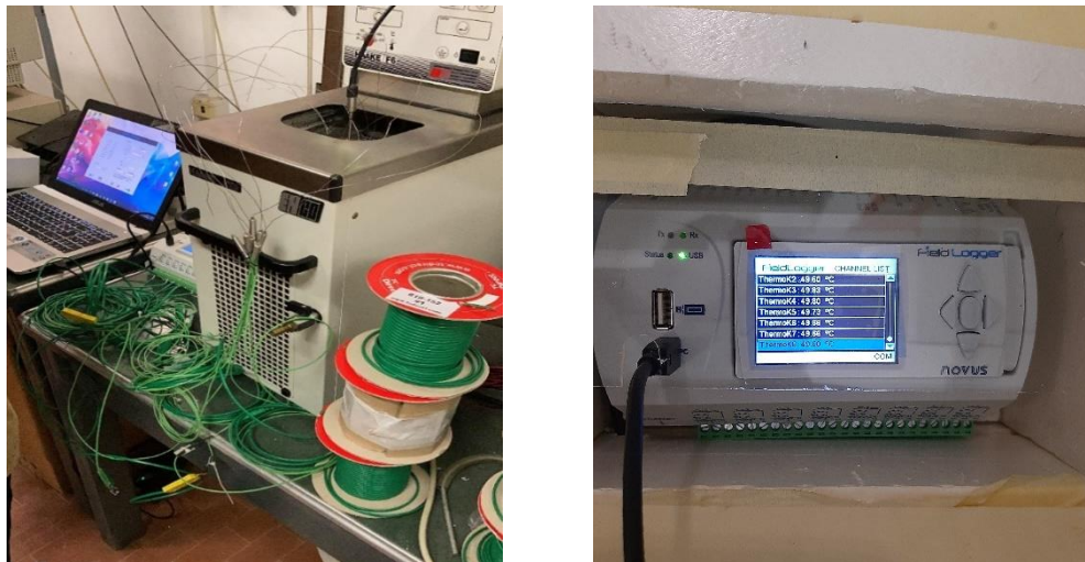
Figure 77. Some steps of the thermocouple calibration process with a thermostatic bath and resistance thermometer.
