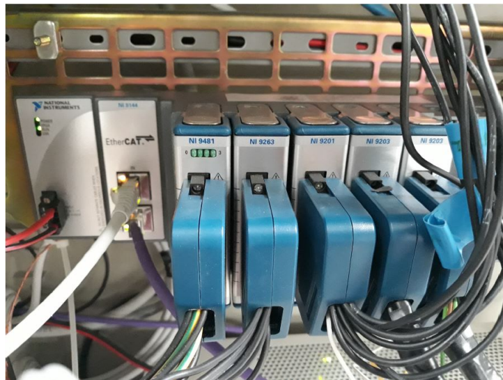
FIGURE 3.21: The first CompactRIO Chassis with its I/O modules.
