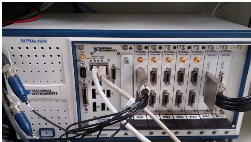
FIGURE 3.18: Cabinet with hardware instrumentation: NI PXIe-1078 chassis with NI PXIe-8135 controller.
