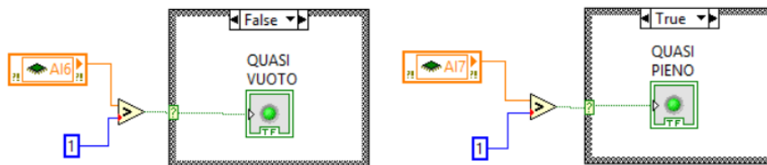
FIGURE 3.33: Block Diagram particular: Analog Inputs from electromagnetic switches of the water level indicator of the tank.
