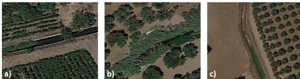
Fig. 4.1 – Orthophoto frames of three different channel portions: (a) flowing water filling the whole cross-section of the riverbed close to the effluent outlet; (b) presence of riparian vegetation indicating a wet stretch; (c) chromatic variation from green to brown suggest a transition from a wet to a dry streambed (Portoghese et al. 2022b).
