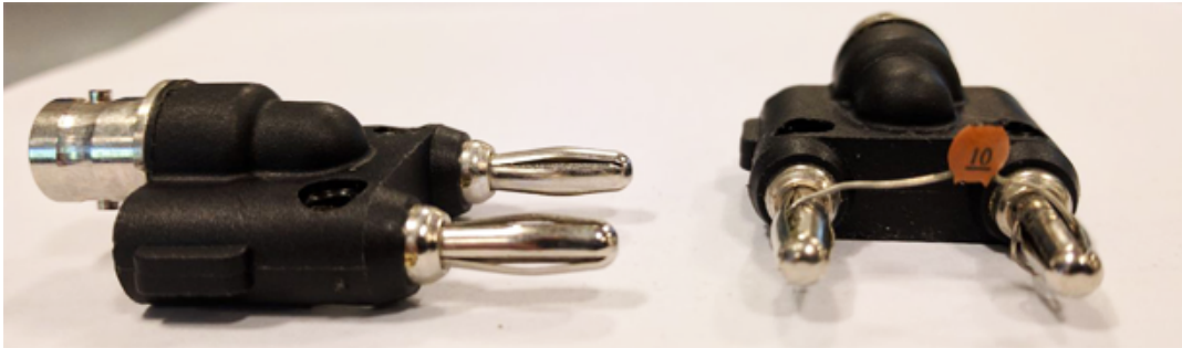
FIGURE 6.11: “F1” (left) and “F2” (right) capacitive fault devices
