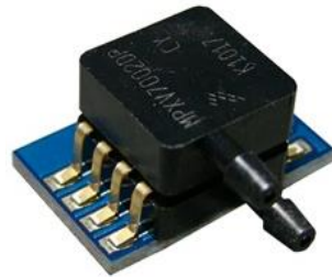
Figure 2.12: Digital Airspeed Sensor
