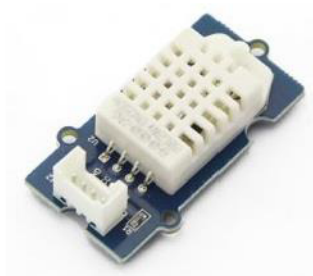
Figure 2.7: Grove - Temperature and Humidity Sensor
