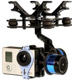
Figure 2.4: Tarot - 2 axes Gimbal GoPro H3
