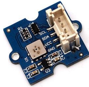
Figure 2.11: Grove - Barometer Sensor
