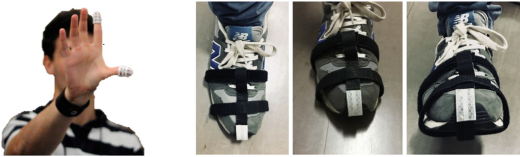
Fig. 4.20 The left image shows a healthy subject wearing the two passive finger markers. The images reported on the right show the foot of a subject doing the foot tapping exercise while he is wearing a passive marker on the toes.
