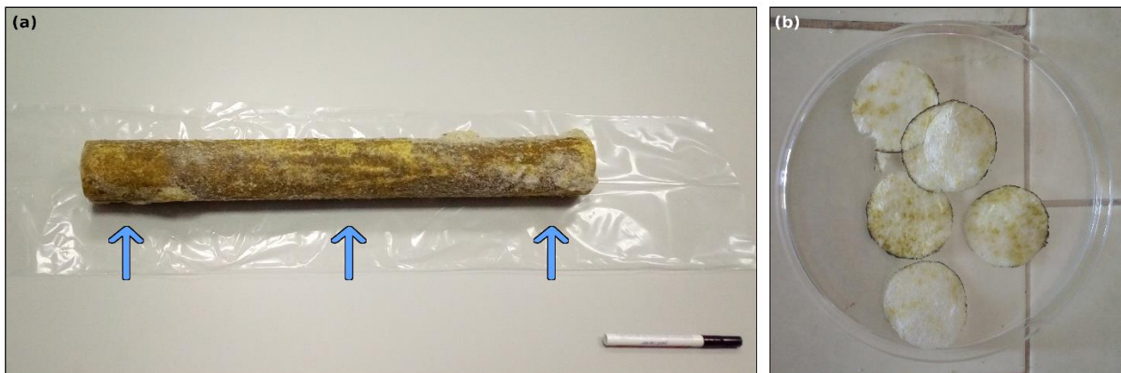
Figure 4: (a) A frozen cartridge filter sampled on February 4th after having filtered ~22.5 hours. The three replicates were sampled from both extremities and the centre (blue arrows). (b) Layers of polypropylene extracted using a cork borer and a pair of heat-sterilized tweezers prior to the DNA extraction. Successively, the layers were cut in half and then in stripes of 1 mm of width. From Cecchetto et al. (2021).
