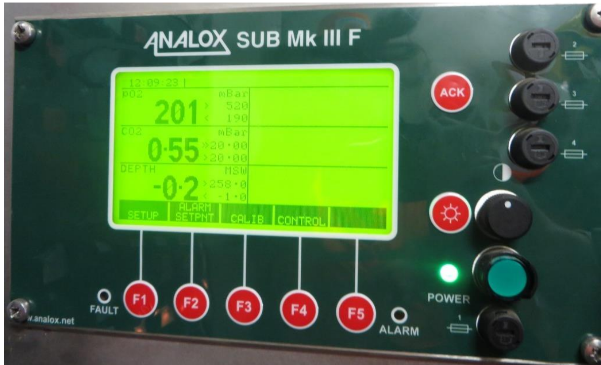
Figure 2-6. ANALOX Atmosphere Monitoring System.
