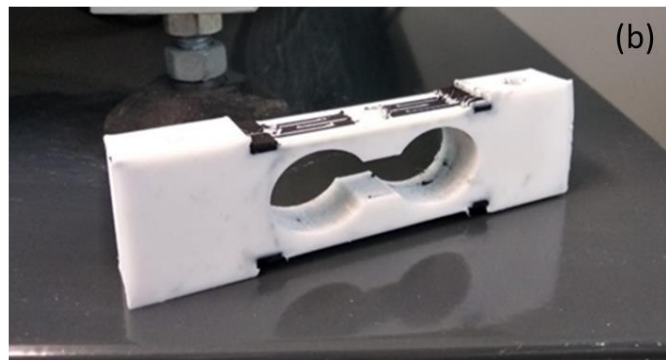
Fig. 2-12- a) load cell in the slicing software, and b) 3D printed load cell with the four embedded strain gauges.
