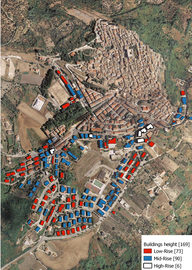
Fig. 14.4 – Heights of RC buildings in Bovino municipality
