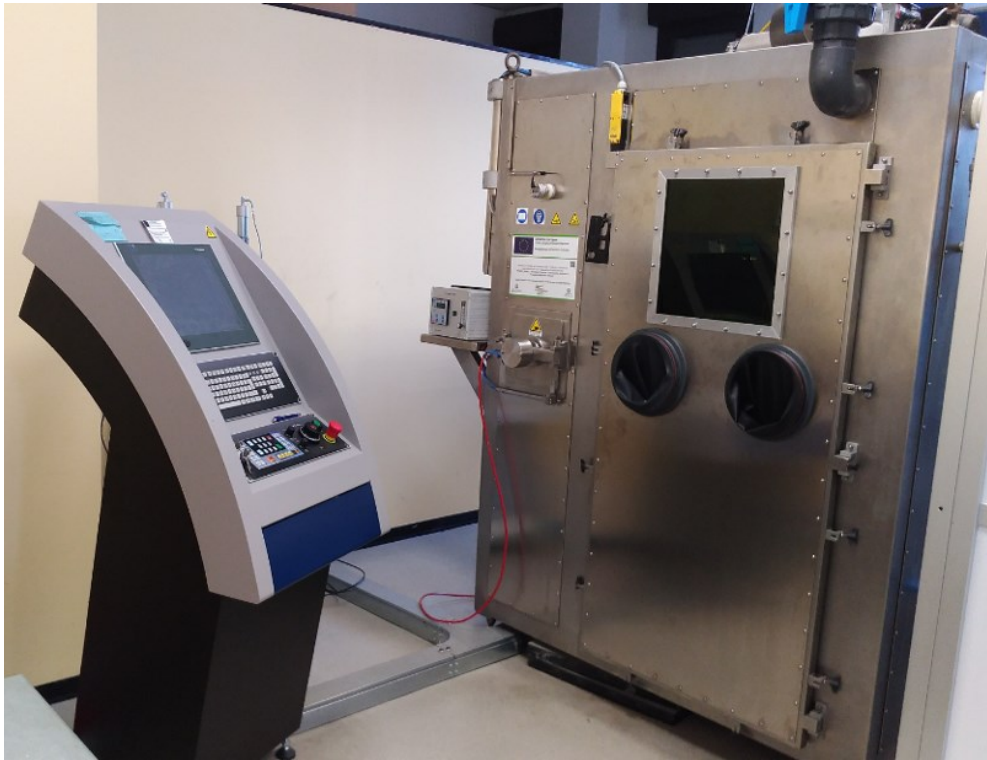
Figure 28 Prototype Direct Laser Metal Deposition system
