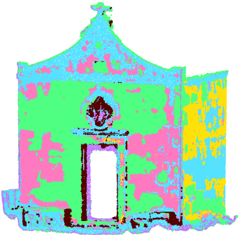
Fig. 67 The classified 2D images re-projected on the 3D model of S.Luigi Chapel
