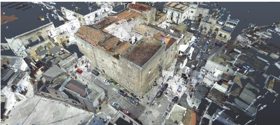
Fig. 80 Merged scan acquisitions in Recap
