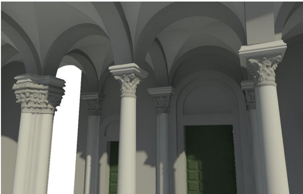
Fig. 35 Meshes of capitals added to BIM model through Dynamo (Ognissanti Church, Italy)
