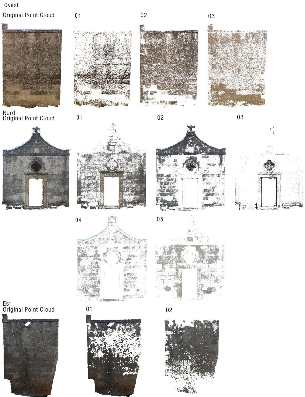
Fig. 53 Clusters in HSV Case 2: Ovest: 01) biological Colonization (23%); 2)moist area (43%); 3) unaltered (34%), Nord:01) moist Area (44%); 02) biological Colonization (60%); 3) deposit/spot (16%); 4) biological patina (48%); 5) unaltered (29%); Est: biological colonization (43%); biological patina (43%).
