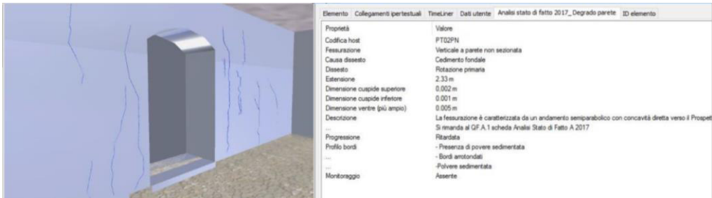
Fig. 98 Correspondence between selected constructional group in the model and the related properties
