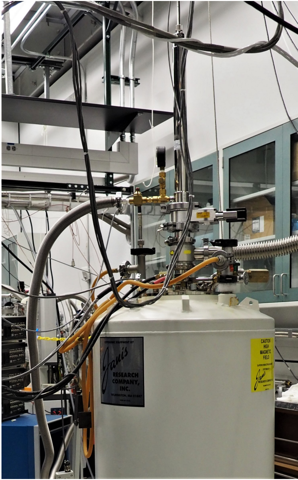
Figure 3.8: Cryogenic system employed for the implementation of the bridge. The system usually works at about 1.5 K and with a magnetic flux density up to 9 T.
