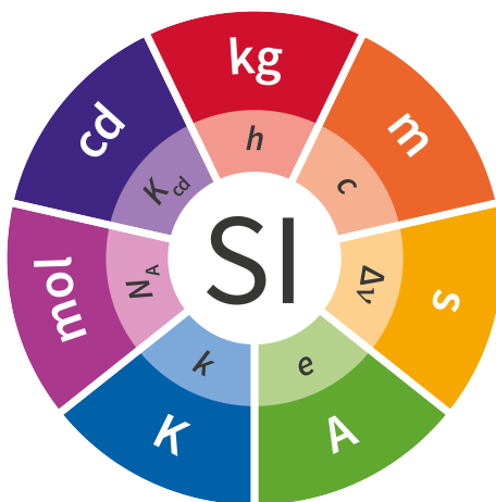
Figure 1.9: The base units of the SI and their defining constants ©BIPM. All rights reserved.
