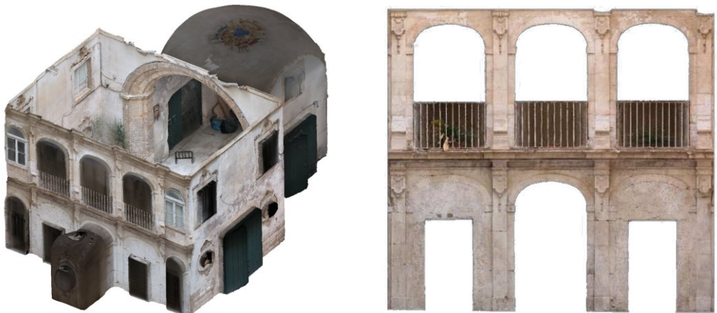
Fig. 34 – High-resolution texturized polygonal mesh of the internal courtyard, with a focus on the lower part of the staircase façade [4],[16].
