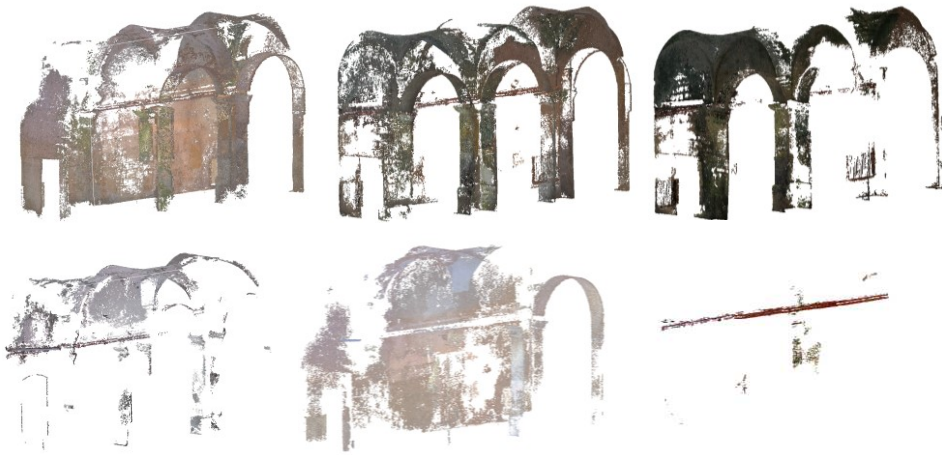
Fig. 72 – Hierarchical segmentation of San Leonardo's cloister in HSV: a) moist area (30%); b) biological patina (27%); c) biological colonization (20%); d) spots/deposit (8%); e) unaltered (11%); f) pipes (1%)
