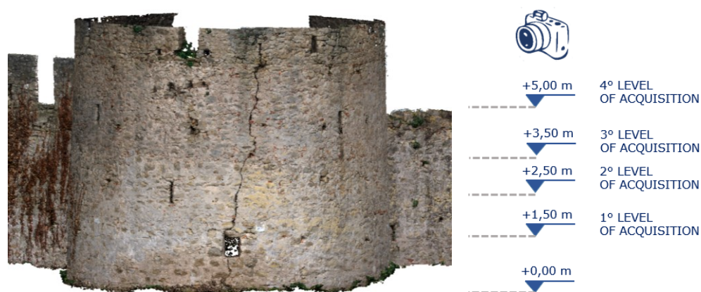
Fig. 93 – Point cloud of the north-tower, with the indication of the points of the four heights of acquisition
