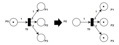
Figure 4.5: Example of parallel transitions.
