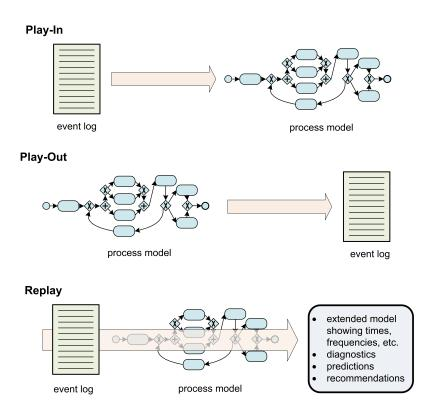
Figure 4.10: Three ways to relate the event log and process models [11].
