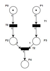
Figure 4.7: Example of synchronous transitions.
