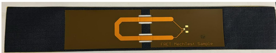
Figure 7-1 FRET latest mechanical samples for material characterization.
