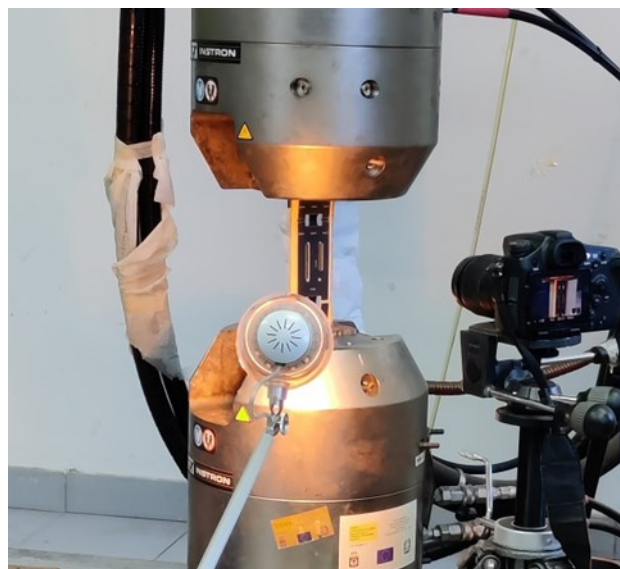
Figure 2-7 Traction test station
