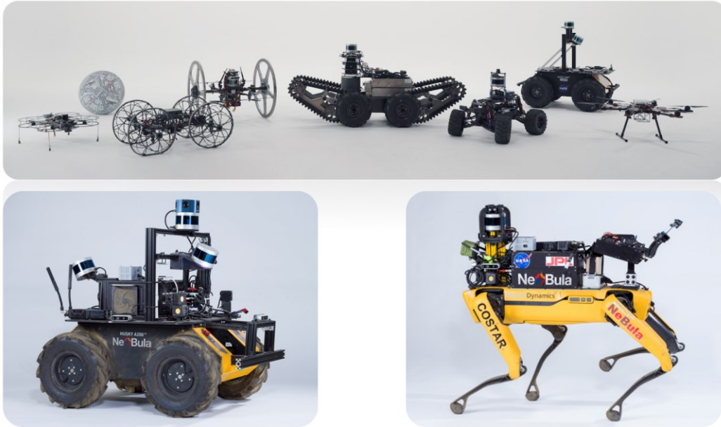
Figure 1-13 – Some of the NASA-JPL CoStar Autonomous and Cooperative Robots
