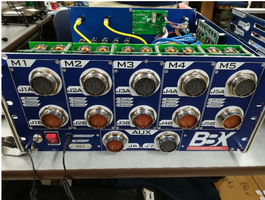
Figure 5-4 Front interface of Blue Box EGSE. Actuator channels are labeled M1 through M5. Top cover removed.
