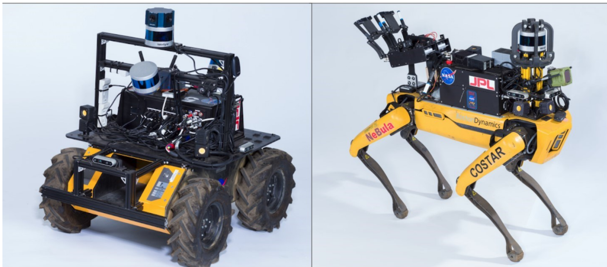
Figure 6-42: NSP equipped on Husky (left) and Spot (right).
