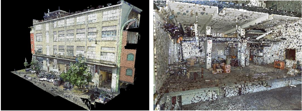
Fig. 74 Voxelisation of the point cloud: external view (on the left) and internal view of the building (on the right).
