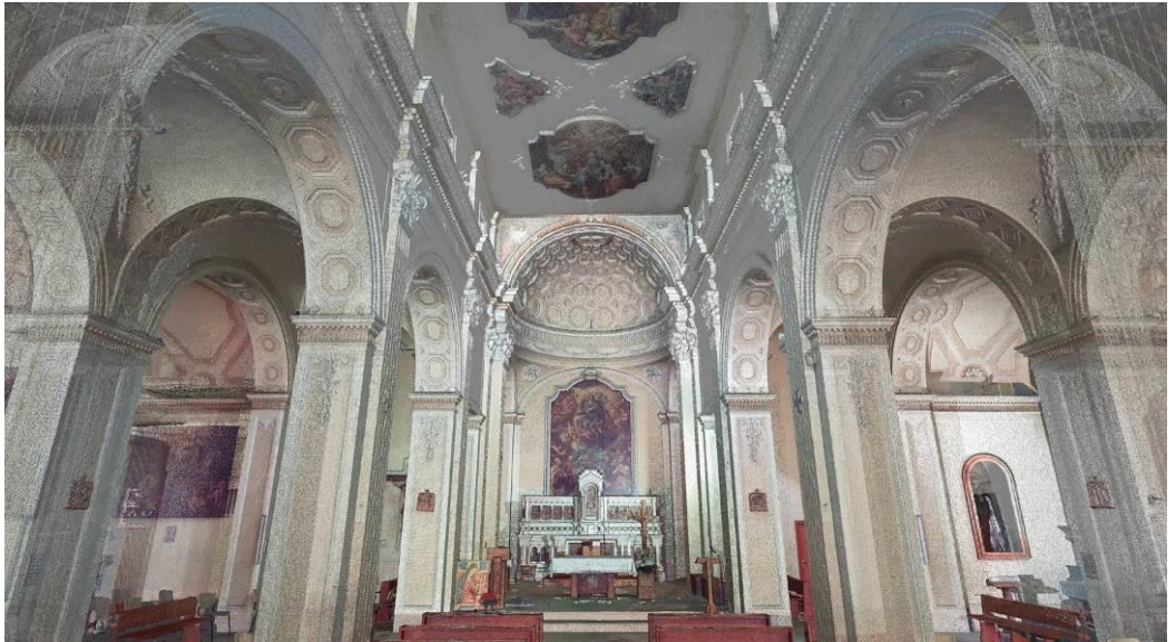
Fig. 18 Range-based point cloud: internal view.
