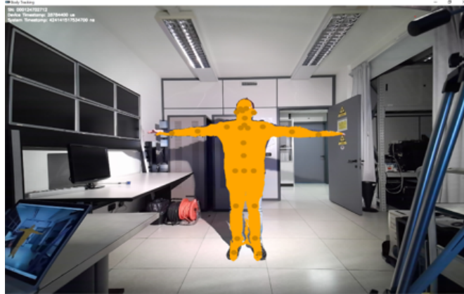
Figure 2.3: Result of body tracking: Sk(N, w/o, 1750, 2) . The orange points represent the estimated positions of the skeletal joints in the 2D image plane.
