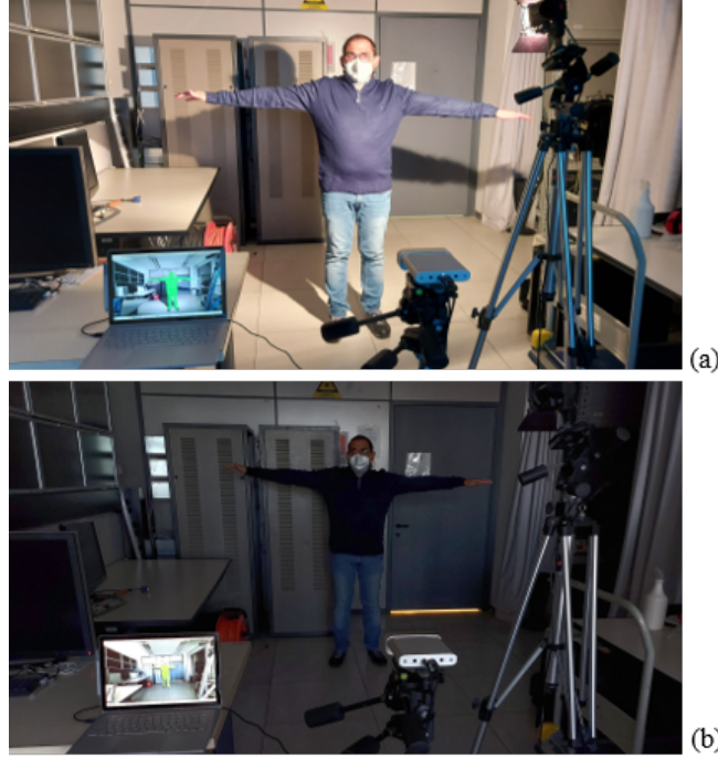
Figure 2.2: Comparison of lighting conditions: (a) E_v = 1750 lux; (b) E_v = 10 lux.
