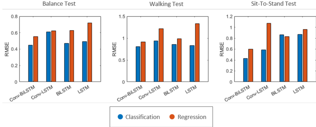
Figure 4.17: Graphs representing the RMSEs values from the Regression Models (orange) vs the Classification Models (blue). Each plot is relative to the exercises within the SPPB test, i.e. BT, WT, and STST.
