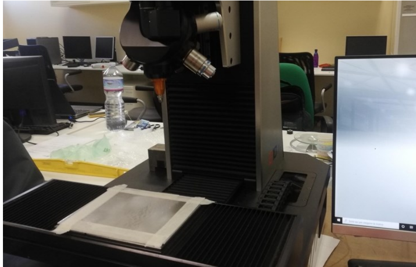
Figure 165. Experimental set-up used for hardness tests.
