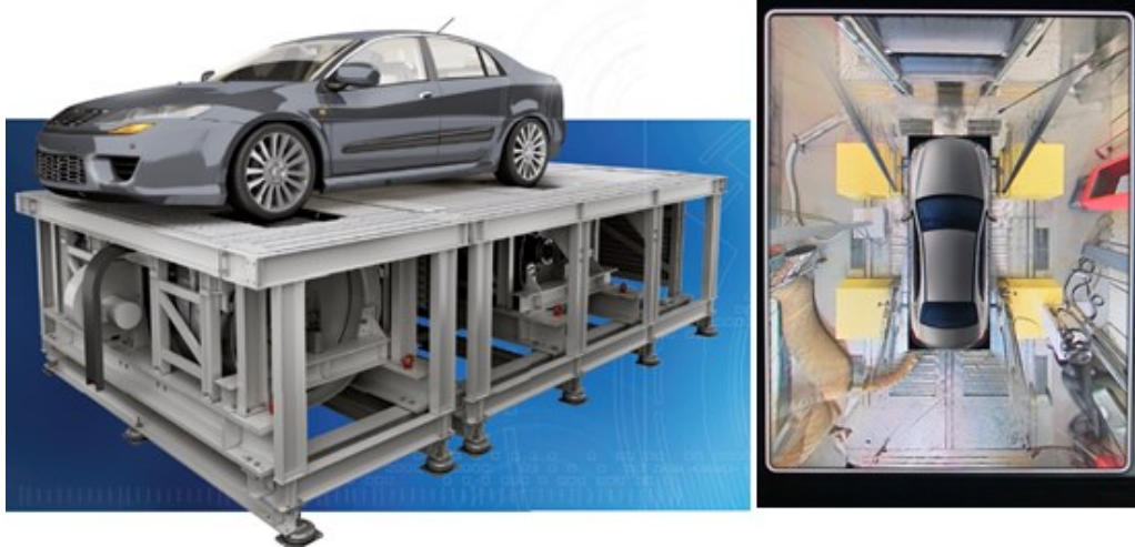
Figure 14: Schematic of Vehicle Installation (left) [49] and real top view (right) on a Chassis-Dynamometer
