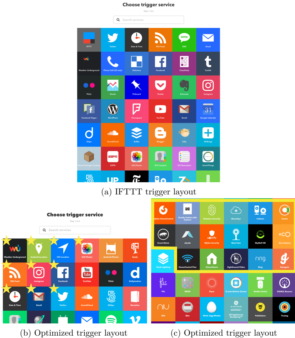
Figure 4.3: A comparison between the trigger layout of IFTTT (a) and the optimized trigger layout calculated by EUDoptimizer with the Simulated Annealing solver (10,000 iterations, (b) and (c)). With respect to IFTTT, in (b) the 10 most frequently used connected entities are placed towards the top of the menu, as indicated by the added stars. Furthermore, the optimized trigger layout is structured in logical groups of entities with functional similarities: in (c), for example, the yellow border highlights a logical group of entities related to home security.
