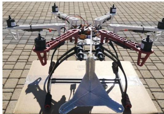
Fig. 42. Example of decoy-UAS during the corner reflector installation.
