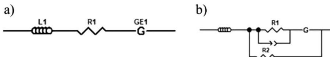
Fig. 1. Schematic representation of the two models used to fit the experimental data obtained in methane. (a) Rs-G model (Mod1); (b) RQ-G with a parallel Rs model (Mod2).
