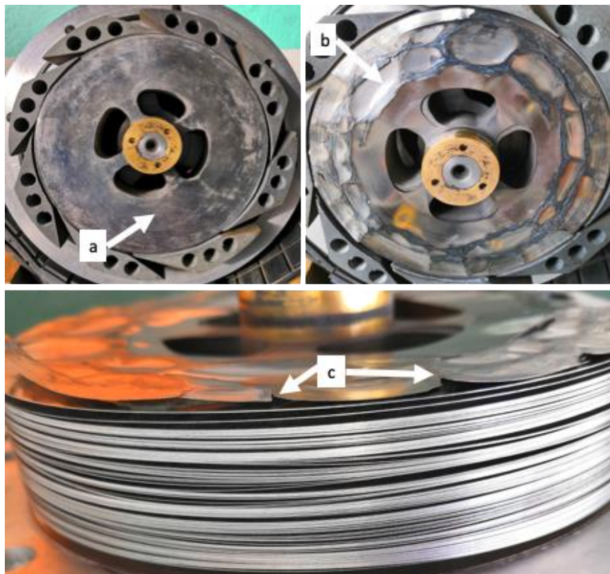
Figure 3.10 Rotor failure at low rotational speeds (a) casing after disk fluttering (b) end disk failure (c) breakage of end disk tip due to hot spot generation
