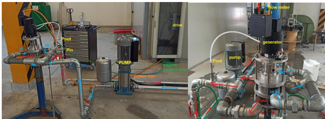
Figure 3.17 Water expander experimental test rig
